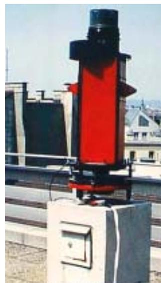
Fig.4: Vienna-Sopron Zenith Camera on its turning plate
