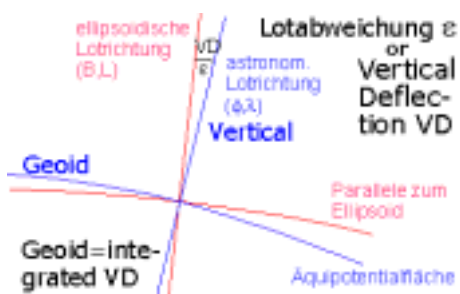
Fig.2: Geoid, ellipsoid coordinates B, L and astronom. Vertical (Deflection VD)
