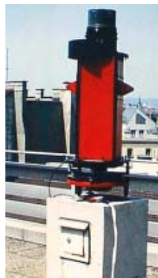
Fig.4: Vienna-Sopron Zenith Camera on its turning plate
