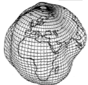
**Fig.1:** smoothed global geoid, based on potential coefficients
